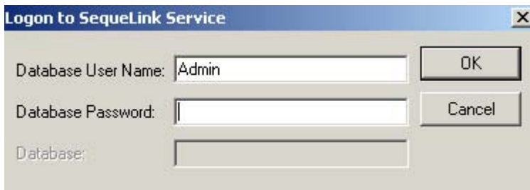
Figure 23: Type the FileMaker file account name and password in the Logon to SequeLink Service dialog box
